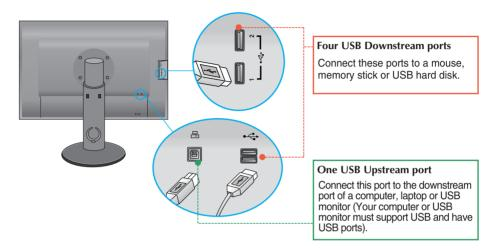
2. The monitor's USB terminal supports USB 2.0 and High Speed cables.
