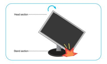
**3.** Be careful with the cables when rotating the screen.
