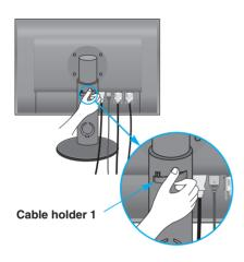
**2.** Please put the power cord and the signal cable in the cable holder 1.
