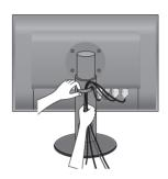
**3.** Please put the power cord and the signal cable in the cable holder 2. While pressing the bottom of cable holder 2 with one hand, pull the top of it with the other hand as shown in the picture.
