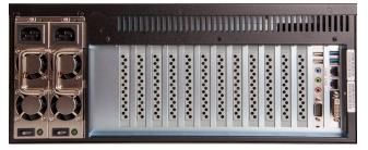
Clarity VCS features server-class CPU, 3rd generation PCIe switched fabric backplane, RAID solid state drives, redundant power suppliers and modular expansion.
