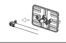
2.Install TRAY to the mount and make sure the KNOB is tightened.
