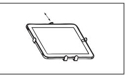
6.Only adjust the single arrow clip to put on or take out the tablet or eReader . Remove device with caution.
