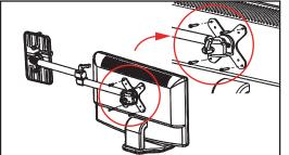
3.Install four screws to four corners VESA base.
