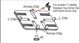
Screw L and ARROW CLIPS onto the TRAY with KNOBS. L Clips can be positioned (top/middle/bottom) to avoid buttons and connectors.
