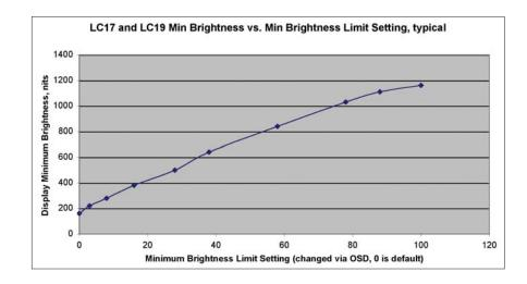
Below is a graph showing the typical minimum brightness limit for a given OSD setting:
