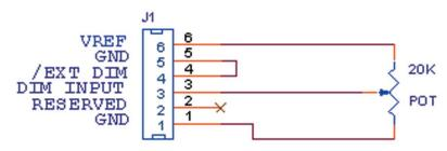
Manual brightness control using a potentiometer
