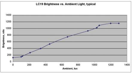
Automatic brightness control with remote photo sensor.
