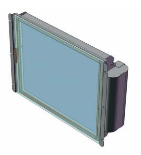
The LC17 and LC19 monitors are available with projected capacitive touch. Projected capacitive is designed to be installed in outdoor applications where rain, splashing liquids, dust, and vandalism are environmental challenges. The sensors are located behind the protective glass layer, whereas traditional capacitive technology employs ITO on the touched surface. Gloved hand use is OK.
