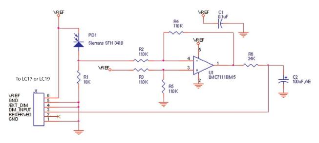
Reference Design for Remote Photo Diode Brightness Control
